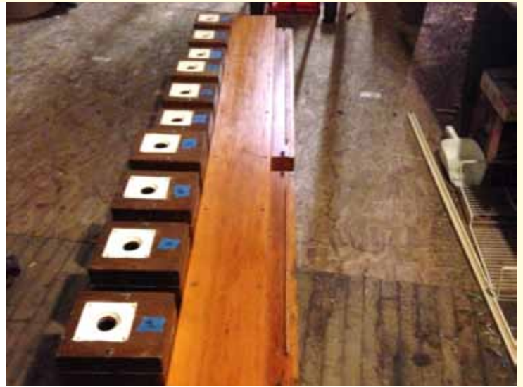
10-note chest ready for placement (photo: Gary Nelson)
